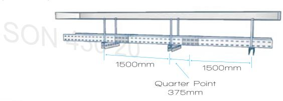
The support span should not be greater than the straight section length to ensure no more than one connector is located between supports. As a general practice, avoid placing connector over supports or at mid-span. However, certain cable tray systems and certain connection plate designs allow for random coupling location.
